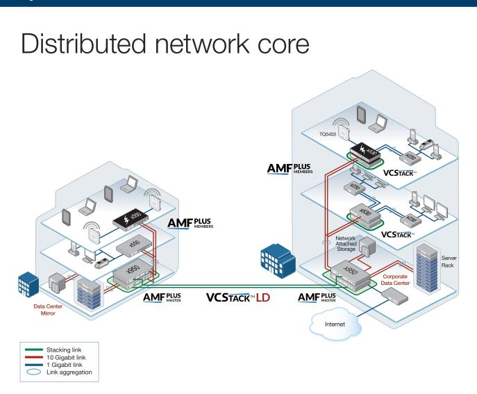
Today's corporate network users demand a high-performing enterprise network that can seamlessly carry multiple converged services, and provide instant access to online resources and applications. This key solution uses the x950 Series and VCStack LD—ideal for a distributed business network core that provides high availability, increased capacity and ease of management.
